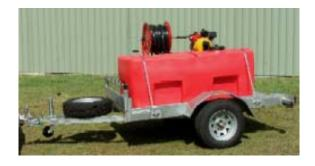
In the interests of safety a new firefighting unit has been purchased capable of delivering 50 litres per minute from its 800 litre tank. Together with its dedicated galvanised trailer both can be rapidly deployed in the event of fire.
