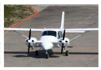
Initially, the concept proved a problem because mounting engines on the wings meant a total wing redesign and the engine pods would obstruct entry to the cockpit. Then the idea came to mount the engines on a short canard mounted on the firewall. Some quick calculations on the weight & balance were not too frightening and it made it possible to get the propellers quite close together to reduce the amount of asymmetric thrust on one engine.
